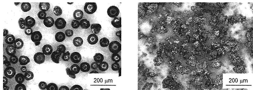
Fig. 1 Typical feature of carbon steel particles and copper particles employed to develop the hybridized particles
