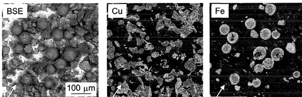
Fig. 2 Scanning electron microscopic images and EPMA elemental maps of Cu and Fe obtained from the “agitated particles”.
