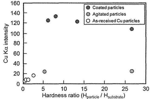
Fig. 8 Cu K $\alpha$  intensity of aluminum substrate with FPP as a function of hardness ratio.
