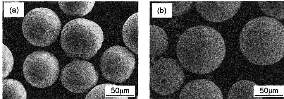
Fig. 3 Typical features of (a) as-received steel particles and (b) the "coated particles".
