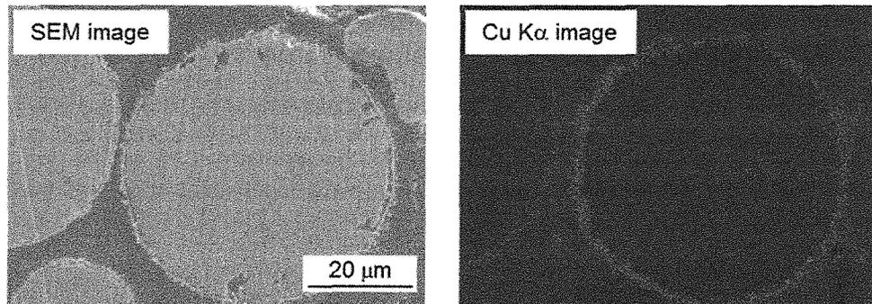
Fig. 4 Cross sectional observation of the "coated particles".
