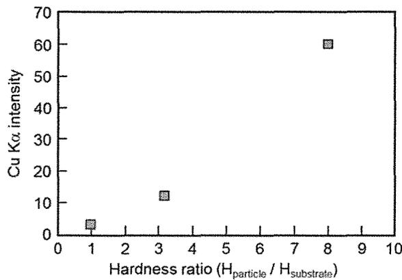
Fig. 7 Cu K $\alpha$  intensity of iron or steel substrate FPP-treated with the "agitated particles" as a function of hardness ratio.
