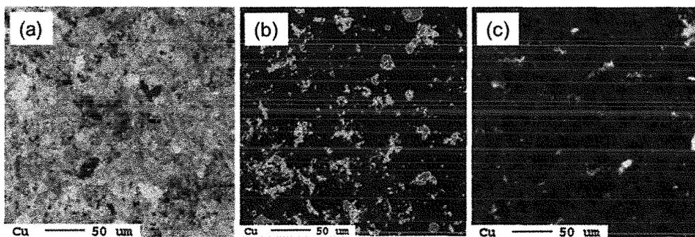
Fig. 5 Elemental map of Cu analyzed by EPMA concerning to FPP-treated 1070 aluminum with (a) "coated particles", (b) "agitated particles" and (c) as-received particles.
