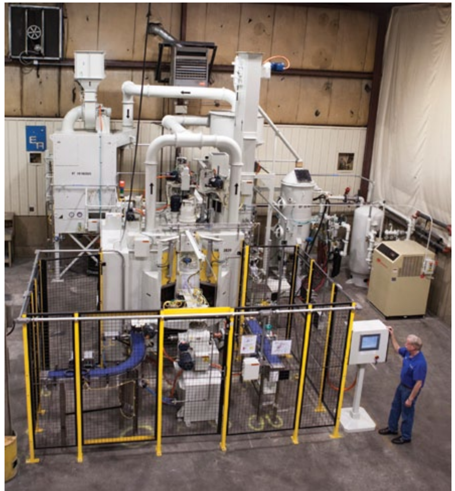
Mike Wern stands by the control panel of an Engineered Abrasives® high-volume index unit with a material handling and robotic system. The machine incorporates EA's patented process to eliminate gear tooth pitting. It will be shipped to a plant in China that builds components for automobiles sold in China.
