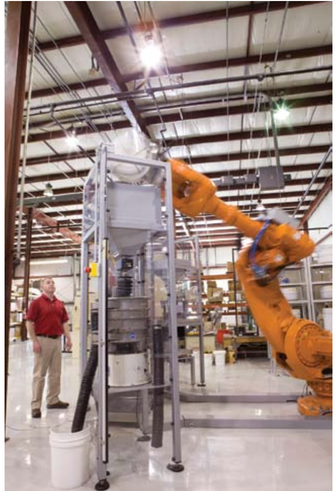
Shotzie, the EI industrial robot, lifts a bucket of media up to a hopper while Bryan Chevie, an EI engineer, watches.
