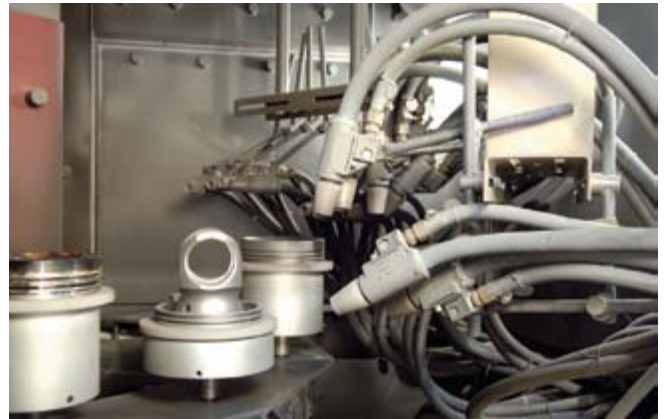
Fig 1. Nozzles targeting specific areas on the component and away from the door.
