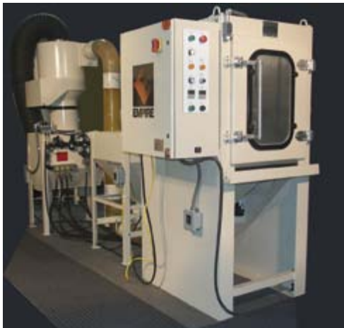
A lip below the access door will reduce media leakage onto the floor.
