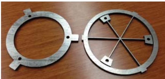
These components of a mirror structure can be rotated very precisely by flexing parts made of a material scientists call "bulk metallic glass." A single point of applied force can rotate the mirror. This technology showcases a use of bulk metallic glasses in space optics. (Image Credit NASA/JPL-Caltech)
