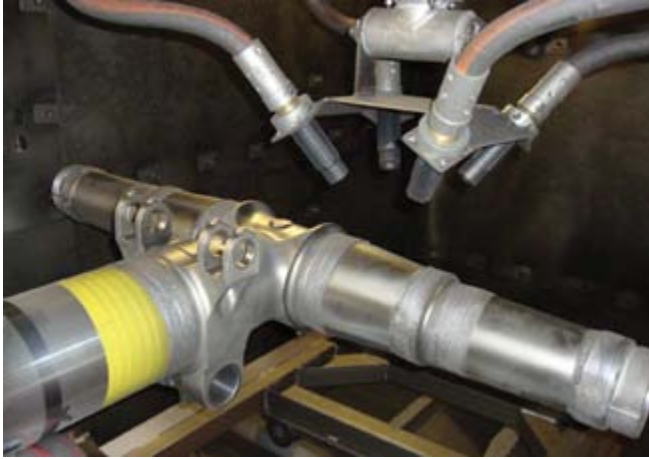
Multi-axis air system for peening landing gear.
