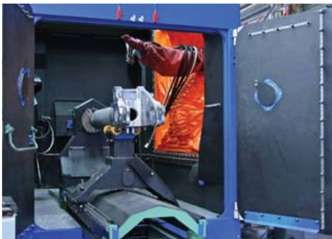
High-accuracy robotic air peening system for landing gear.
