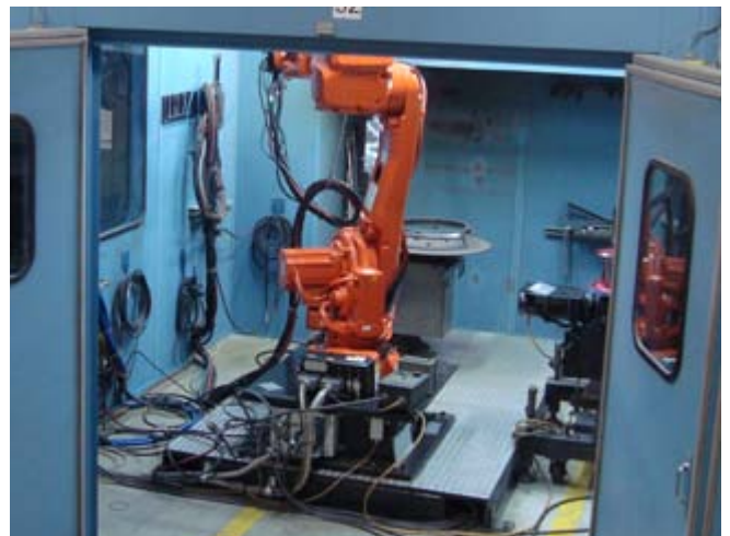
Robot for applying thermal spray coating.
