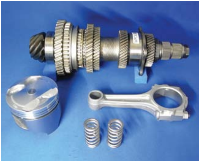
Figure 2. A piston, automotive gear, connecting rod and coil spring that have received the WPC treatment. The MoS 2 shot process was applied to the piston skirt.
