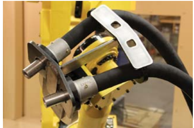
Pressure blast nozzles mounted on a robotic arm provide travel path flexibility
