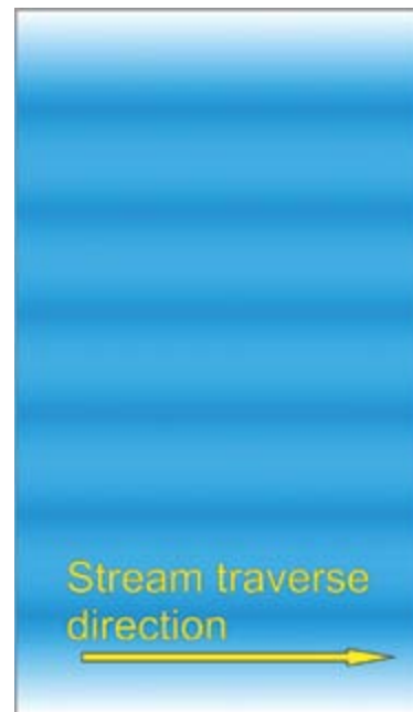
Fig.7. “Stripe” effect of coverage induced by overlapping linear passes.
