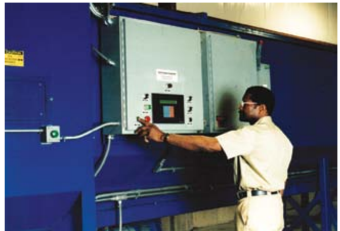
For a number of years, Blackman was responsible for a dedicated, 80 foot-long machine that shot peened 32 foot-long drill pipes (ID and OD) used for oil and gas exploration.
