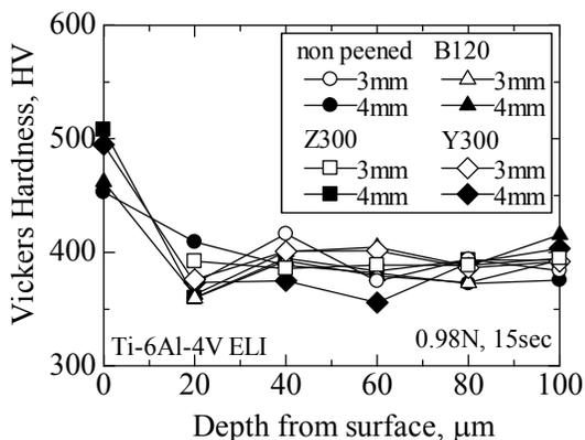
Fig.5 Vickers hardness distributions.
