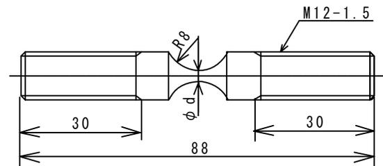
Fig.3 Configuration of fatigue specimens, mm.
