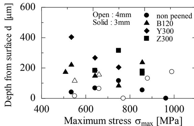
Fig.9 Depth of crack initiation sites.
