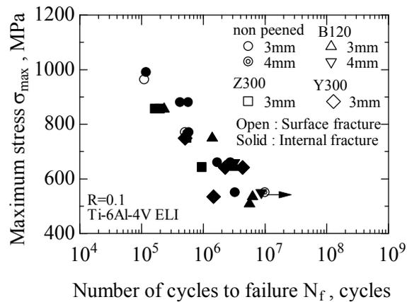
Fig.7 S-N diagram of axial loading fatigue results.
