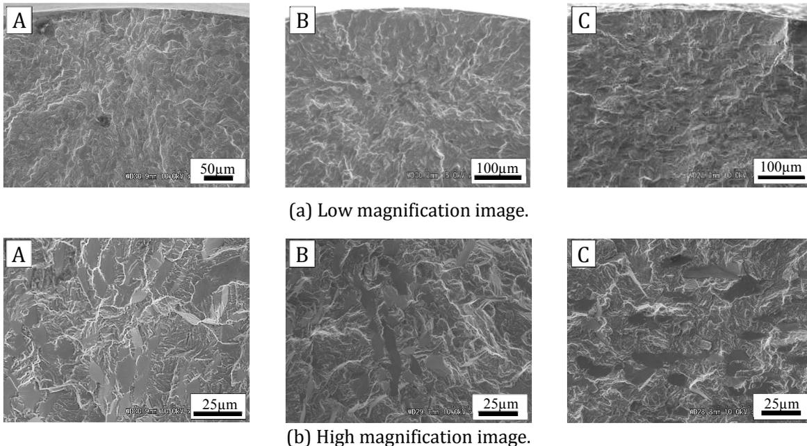
Fig.8 Fracture surface of the axial load fatigue test. (A) 3mm non peened (749 MPa,  $5.83 \times 10^5$  cycle), (B) 3mm Y300 (642 MPa,  $4.32 \times 10^6$  cycle), (C) 3mm B120 (535 MPa,  $6.26 \times 10^6$  cycle)
