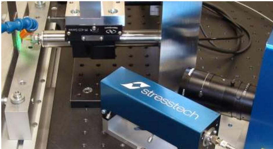
Figure 1 Example of the measurement setup of the ESPI system, left to right: illuminated sample, electric drill on orbiting device, illumination stand, camera.
