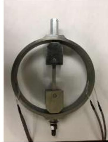
**Figure 3:** Photo of proof ring-based load cell used to apply a tensile load in-situ during the x-ray diffraction experiments. The same load cell was used with both the  $\sin^2\psi$  and  $\cos\alpha$  measurement methods.
