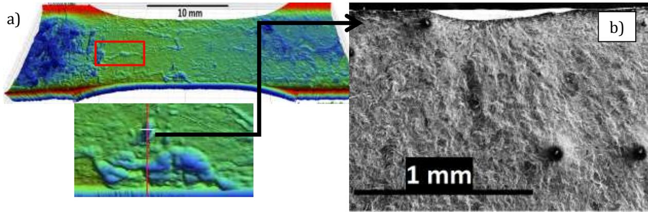
**Figure 2:** a) Surface scan of an as-forged specimen showing the crack initiation site and propagation, b) Fatigue failure surface of the same specimen showing the large defect in which the crack initiated
