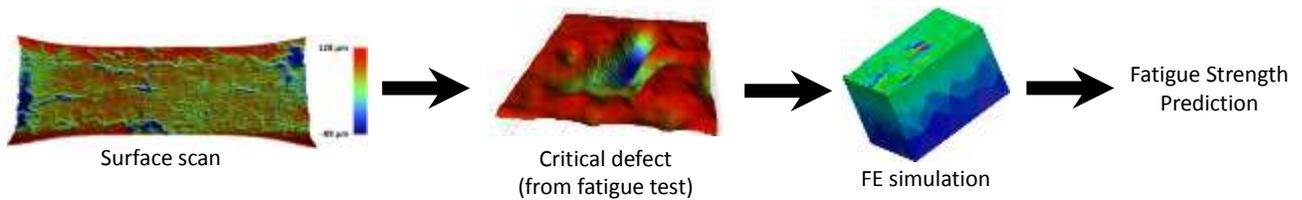
Figure 4. Process for performing the FE simulations of the critical defects.
