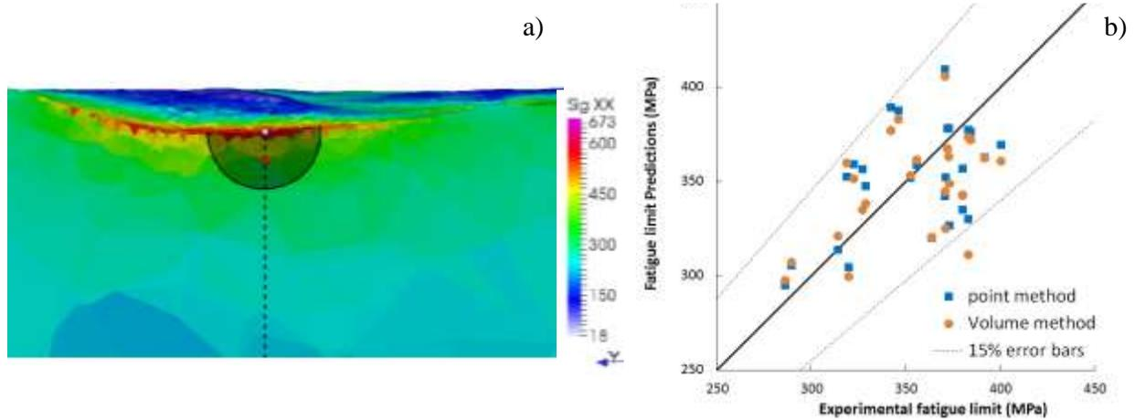
**Figure 5.** a) Cross-section of the FE simulation of the critical defect in figure 2. Stress values are in MPa, the white dot locates the maximum stress. The point method (red dot) and volume method (sphere centered on the white dot) are indicated, b) Predictions for each method
