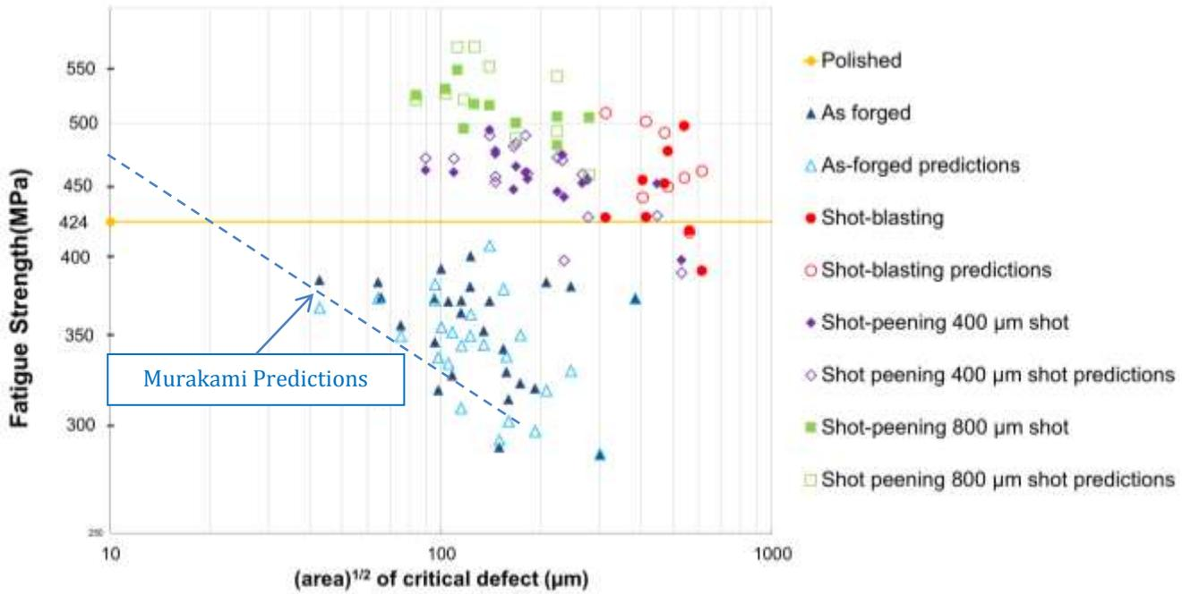
Figure 3. Kitagawa diagram of the fatigue tests, with fatigue strength and critical defect size
