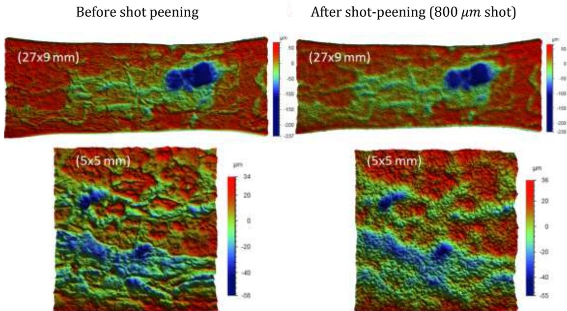
**Figure 1.** Surface scan of an as-forged specimen, before and after shot-peening
