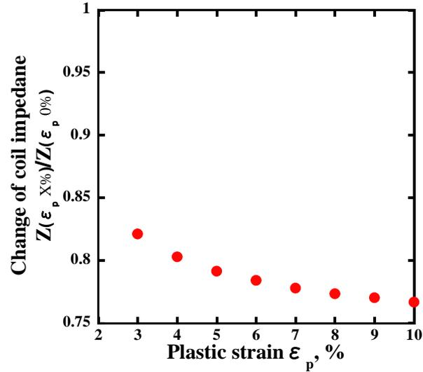
Figure 4 Effect of amount of the plastic strain on the coil impedance at 5902 Hz.
