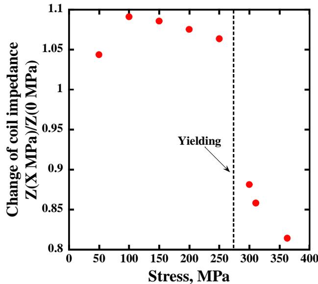
Figure 3 Coil impedance measurement result of 5902 Hz during loading the specimen.
