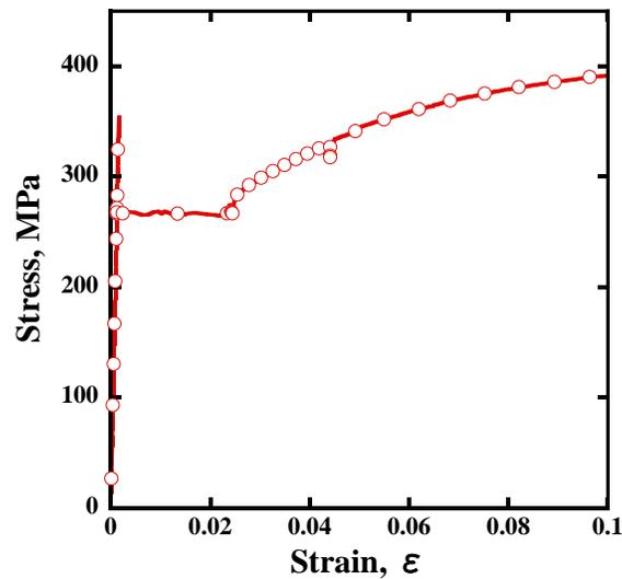
Figure 2 Stress-strain curve of the mild steel used in this study.
