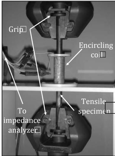
Figure 1 Experimental apparatus used in this study.
