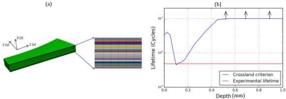
Figure 5: Fatigue simulations after shot peening. (a) Mesh discretization to introduced the residual stress profiles for SP1 conditions at  $N_f/2$  (b) Fatigue life time prediction at 600 MPa ( $R=-1$ ) vs the depth of the specimen (1 mm = mid-thickness) using Crossland criterion compared to experimental data.
