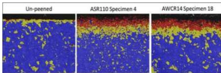
Figure 3 - Grain misorientation maps for un-peened and peened specimens
