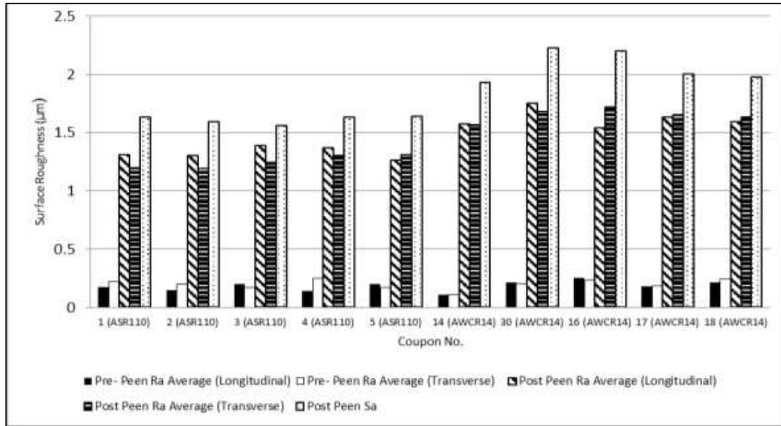
Figure 1 - Comparison of surface roughness results for IN718 specimens peened with ASR110 & AWCR14
