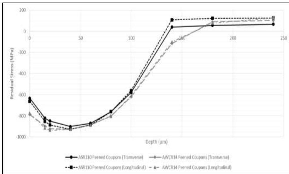
Figure 2 - Averaged residual stress profiles for IN718 Peened with ASR110 & AWCR14
