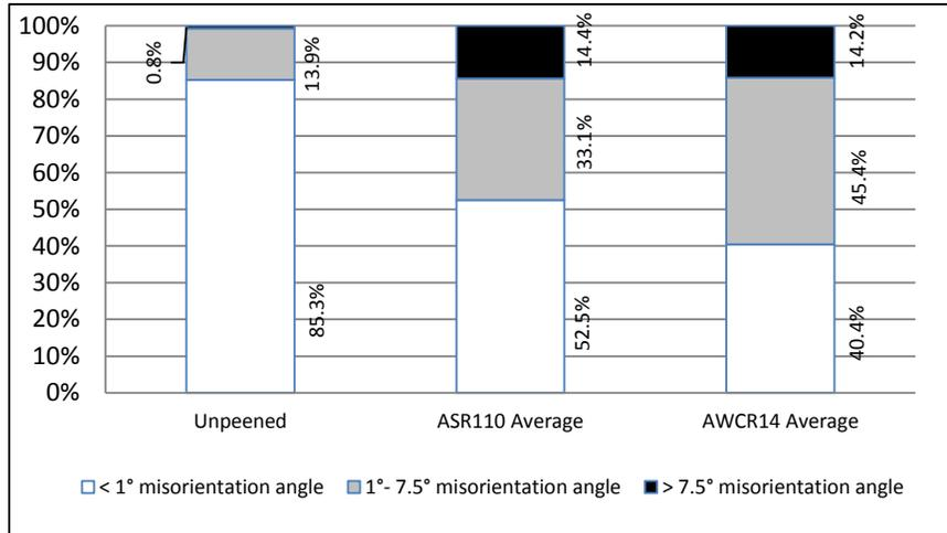
Figure 4 - Grain misorientation percentages for un-peened and peened specimens
