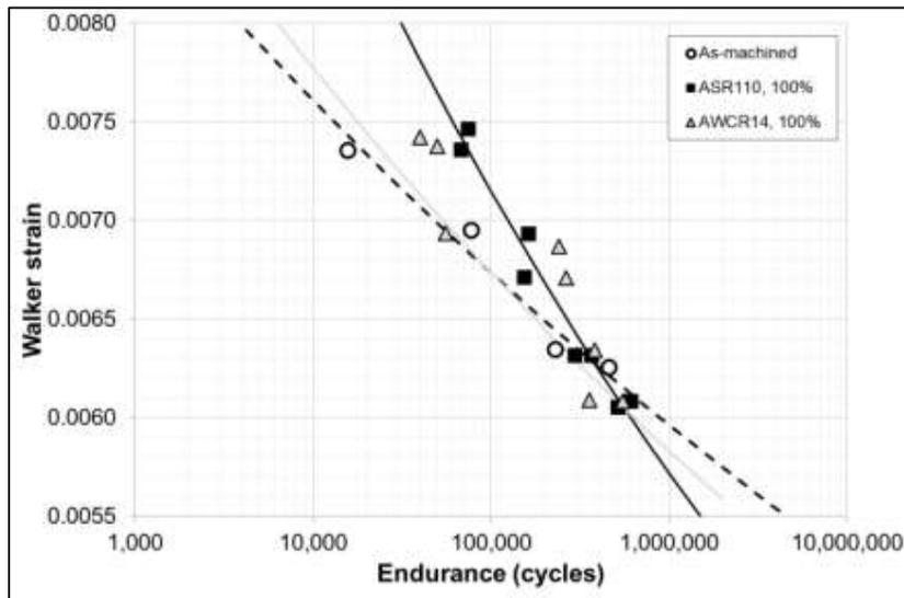
Figure 5 - Fatigue test results for un-peened and peened specimens
