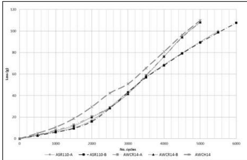
Figure 6 - Durability test results for ASR110, AWCR14 & AWCH14 media
