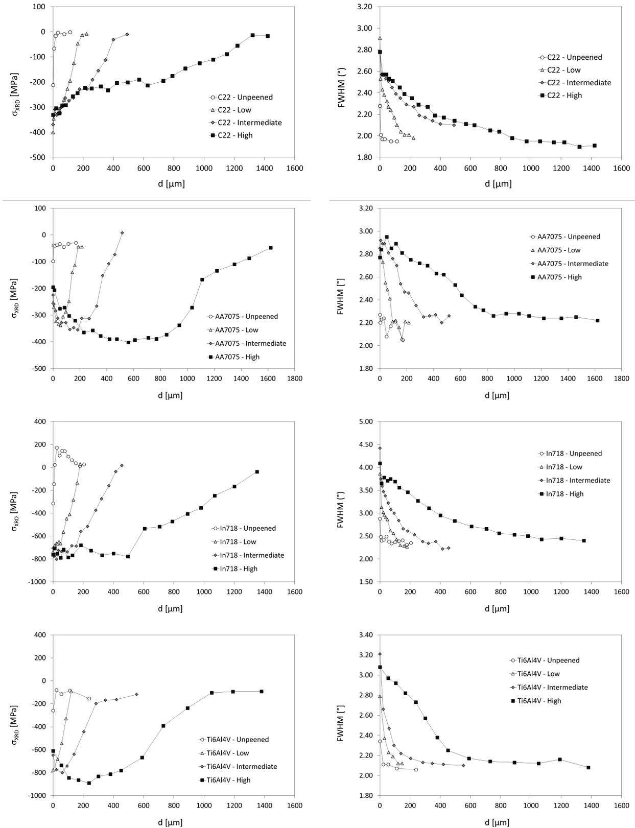
Figure 1: Incremental XRD characterization after SP. Left: residual stress, right: FWHM. From top to bottom: C22, AA7075, In718, Ti6Al4V.
