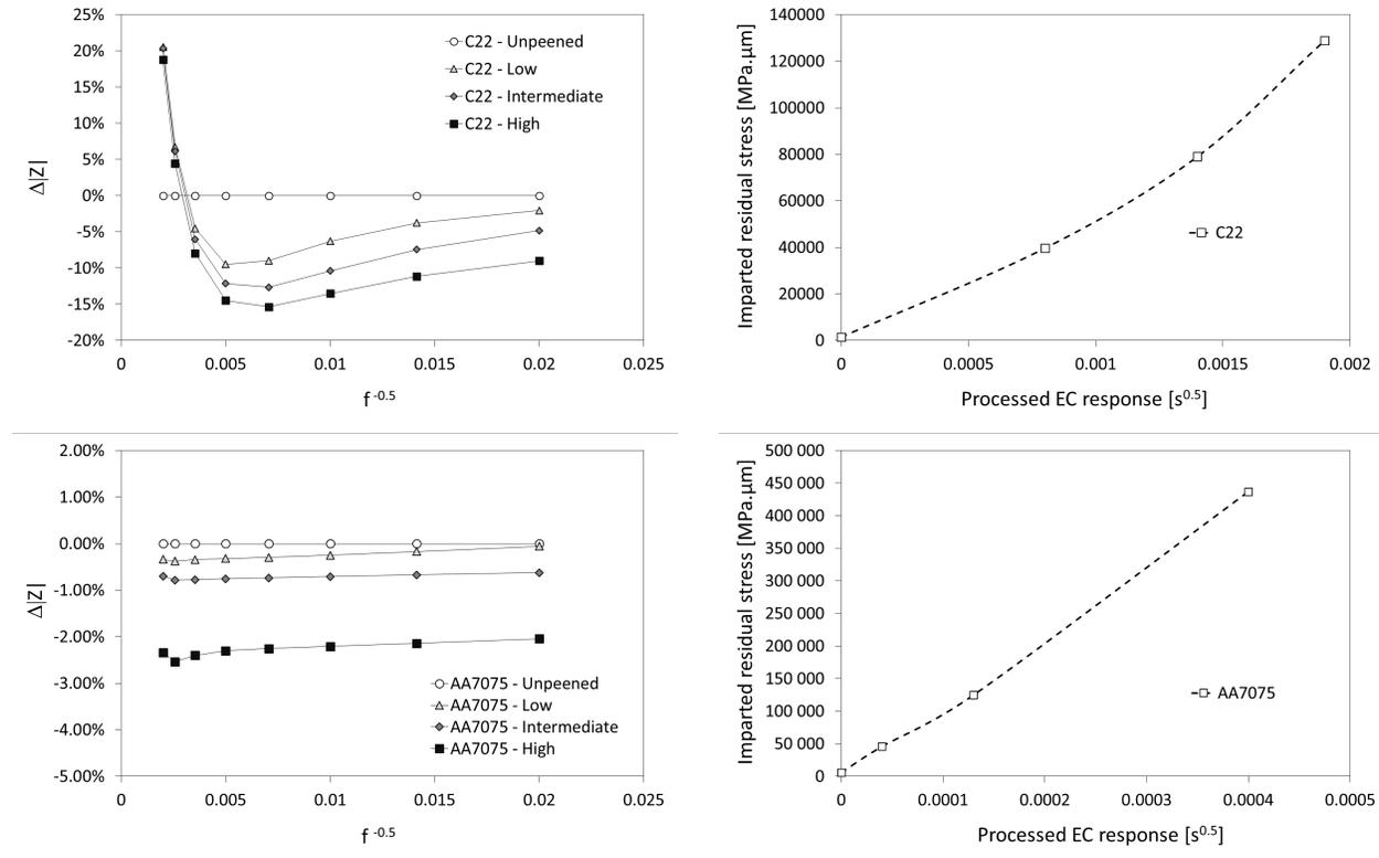
Figure 3: Change in the magnitude of the impedance caused by shot peening (left), and correlation between the multifrequency EC test response as processed in the present paper and the XRD residual stress profile surface area, namely imparted residual stress (right). Results for C22 (top) and AA7075 (bottom).
