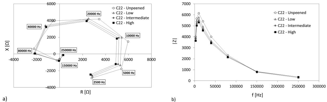
Figure 2: Coil impedance  $Z$  on the complex plane (a) and magnitude of the impedance  $|Z|$  vs. frequency  $f$  (b) for C22 steel samples
