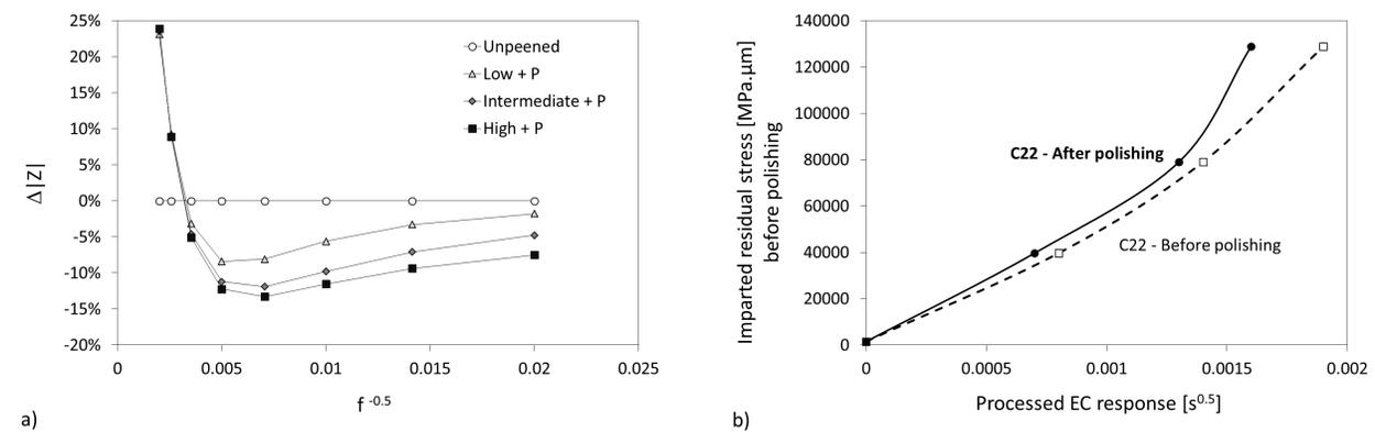
Figure 4: Effect of polishing the SP-induced roughness on EC response
