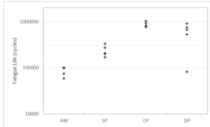
Figure 1: Fatigue life of peened Al-Cu-Li specimens
