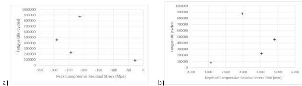
Figure 5: Fatigue life as a function of residual stress parameters – a) peak compressive residual stress, b) depth of compressive residual stress field
