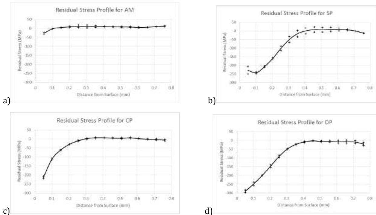
Figure 2: Residual stress profiles - a) As-Machined + anodized, b) Conventional steel media shot peened + anodized, c) Ceramic media shot peened + anodized, d) Duplex conventional steel media followed by ceramic media peened + anodized.
