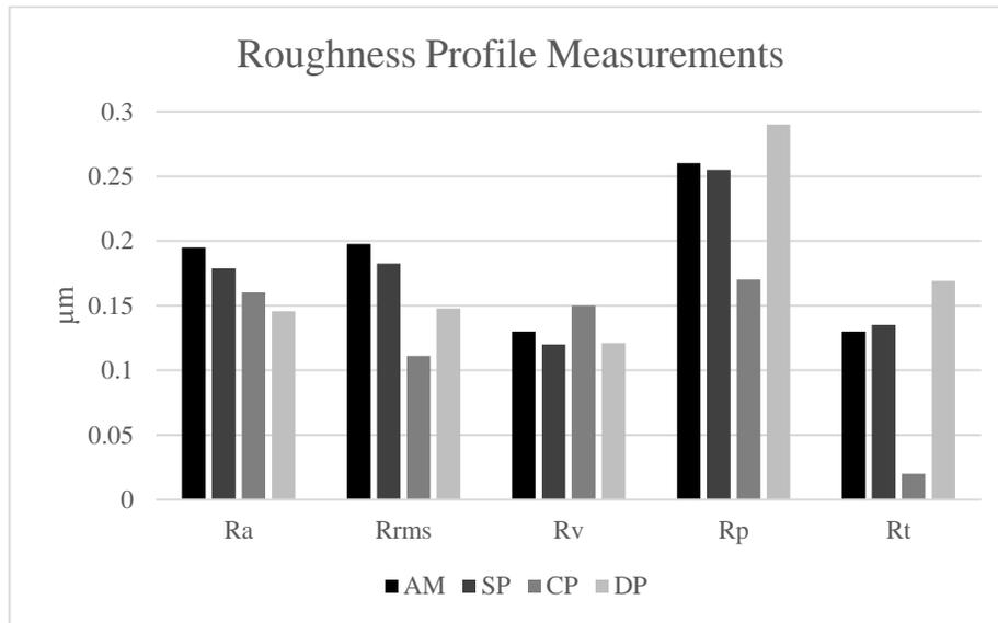
Figure 3: Surface roughness measurements for different peening conditions
