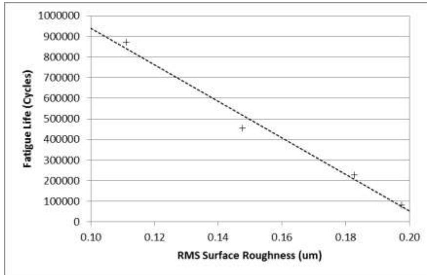
Figure 4: Fatigue life as a function of specimen surface roughness
