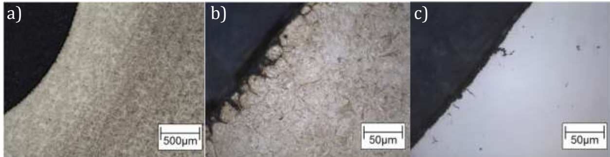
Figure 2: microstructure before shot peening (initial condition): a) overview of the tooth root in etched condition and b) near surface zone in etched and c) not etched condition
