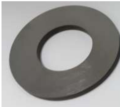
Figure 1 Photo of a rolling contact fatigue specimen
