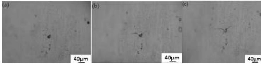
Fig. 1 Replica SEM images showing small crack growth in an un-peened specimen of 7475-T7351 aluminum alloy for N cycles: (a) N = 3000; (b) N = 6000; (c) N = 9000 [4].
