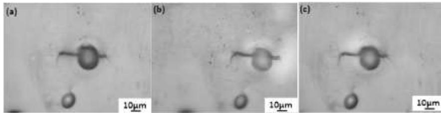
Fig.2 Replicas SEM images showing small crack growth in a shot peened specimen of 7475-T7351 aluminum alloy for N cycles: (a) N = 6000; (b) N = 7000; (c) N = 8000 [4].
