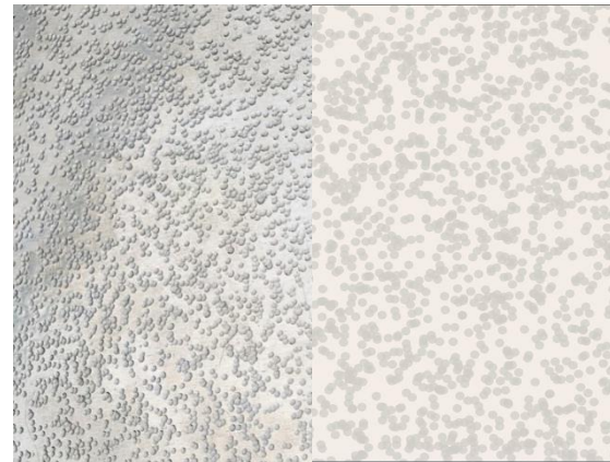
Pict. 11: Aluminium surface after 50% coverage; real microscope picture (left) and artificial picture from the software (right).
