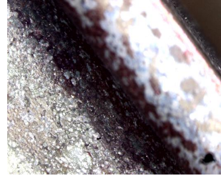
Pict. 1: microscope picture of the internal beam radius of a con'rod. Despite the surface was covered, before peening, with red marker for whiteboard, the geometry makes the coverage evaluation difficult.
