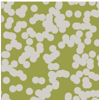
Pict. 4: 50% coverage, simulating 0.600 mm cut wire shot, as new.
