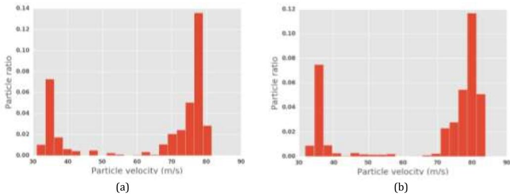
Figure 6 Peen velocity histogram at measurement plane from (a) OpenFOAM and (b) ANSYS-FLUENT
