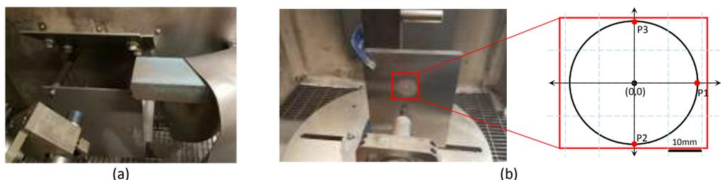
Figure 2: (a) Shot velocity measurement set-up (b) Set-up for coverage assessment and coverage assessment on plate
