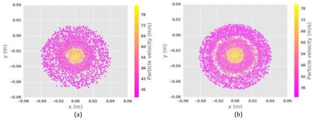
Figure 7 Distribution of peens on the substrate surface: (a) OpenFOAM® and (b) ANSYS-FLUENT
