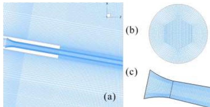
Figure 4: Mesh at the mid-range cutting plane in the span-wise direction. (a) nozzle and zone around the nozzle until the workpiece (b) entrance of the nozzle (c) enlarged part of the nozzle
