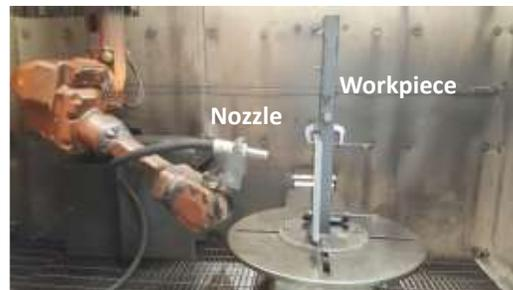
Figure 1: Shot peening experimental setup
