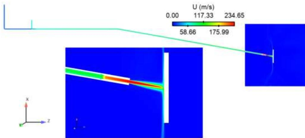
Figure 5 Gas flow velocity contour at the middle range cutting plane
