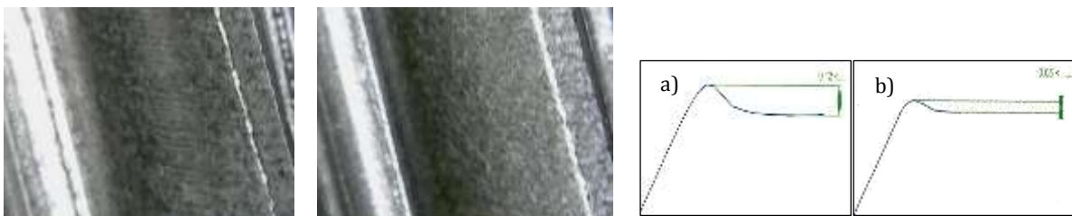
Fig. 6 – Gear flank before and after shot peening and measurements: a) before and b) after shot peening
