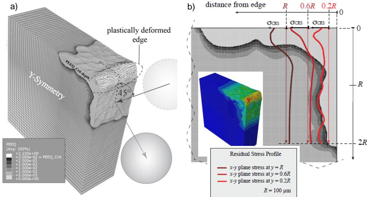
Fig.5. PEEQ, damage induced and residual stresses over a representative 3D edge feature.
