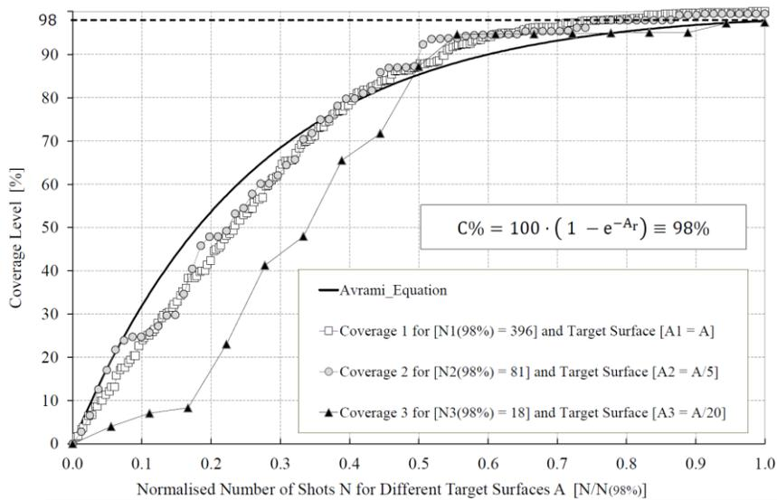
Fig.2. Coverage of shot peening following Avrami definition for three different analyses.
