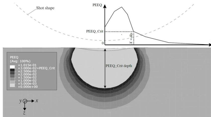
Fig.3. PEEQ under a single shot model.
