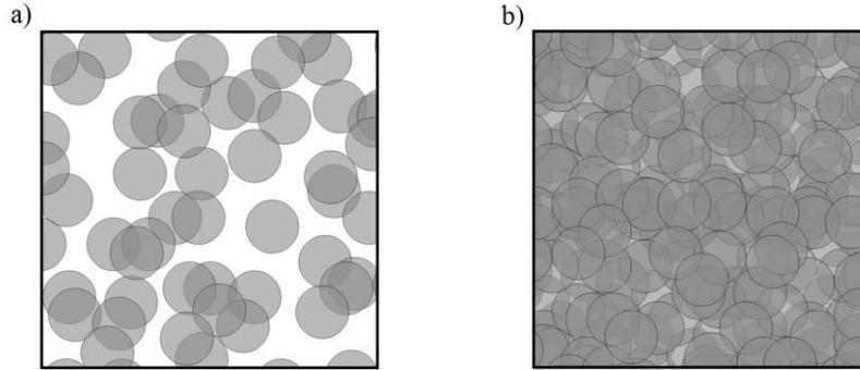
Fig.1. Progression of coverage of shot peening.
