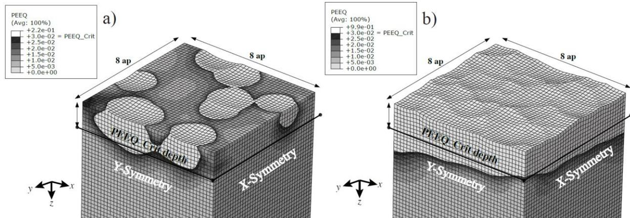
Fig.4. PEEQ evolution for a symmetry cell model.
