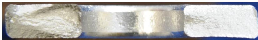
(b) Cavitation peened specimen, t_p = 5 s/mm, \sigma_{max} = 170 MPa, N = 7.04 \times 10^5
