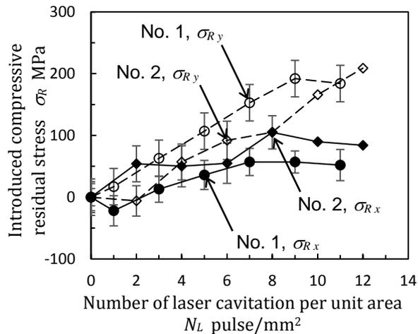
Fig. 6 Introduced compressive residual stress as a function of number of laser cavitation per unit area
