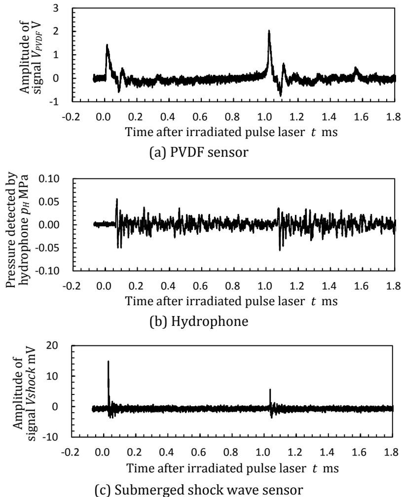
Fig. 5 Output signal from sensors
