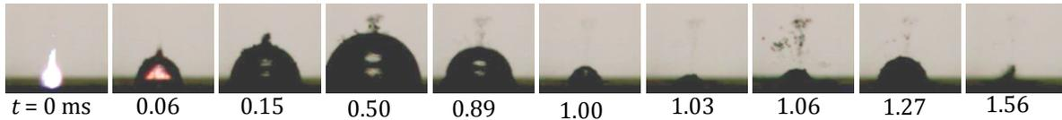
Fig. 4 Aspect of laser abrasion and laser cavitation
