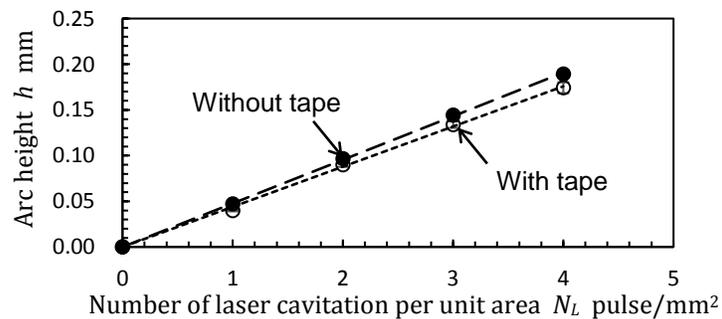
Fig. 3 Peening intensity measured by Almen strip of A-gage
