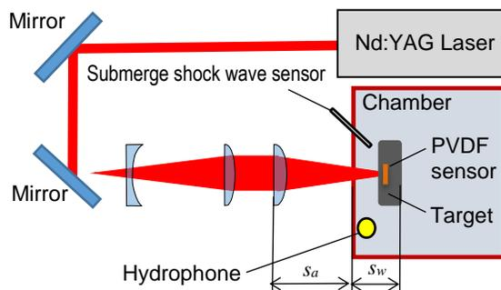
Fig. 1 Schematic diagram of cavitation peening system using laser
