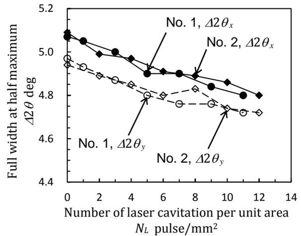
Fig. 7 Decrease of full width at half maximum as a function of number of laser cavitation per unit area
