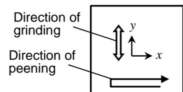
Fig. 2 Direction of laser peening and direction of stress
