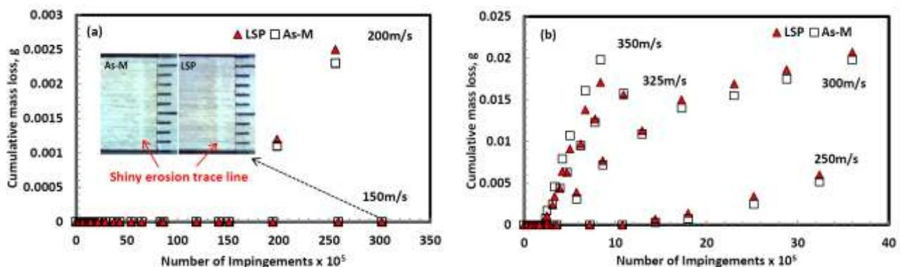
**Figure 3.** WDE curves for As-M versus LSP at (a) 150-200m/s and (b) 250-350m/s.
