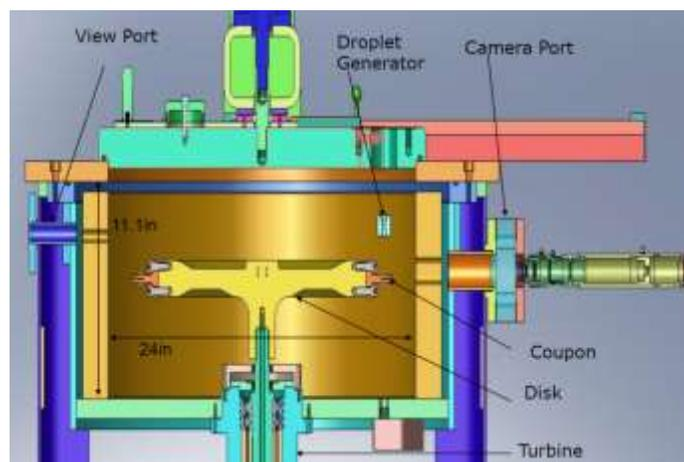
**Figure 2:** Schematic illustration of the water erosion rig used in the present work.
