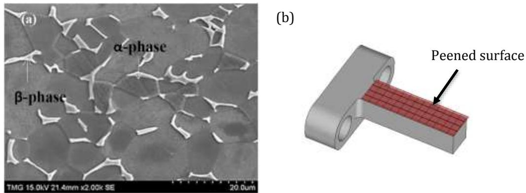
**Figure 1:** (a) initial Ti-6Al-4V microstructure and (b) typical T-shaped flat sample machined.
