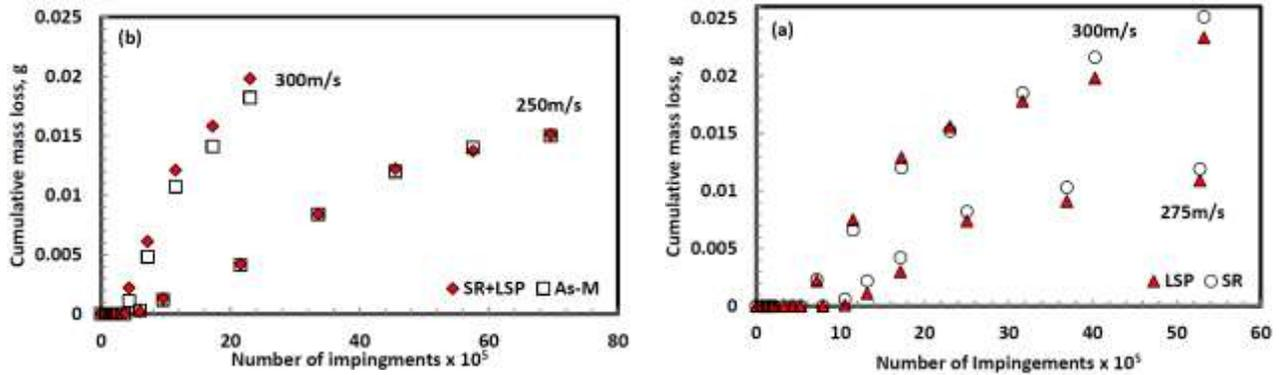
**Figure 4:** WDE curves for (a) SR versus LSP and (b) SR+LSP versus As-M.
