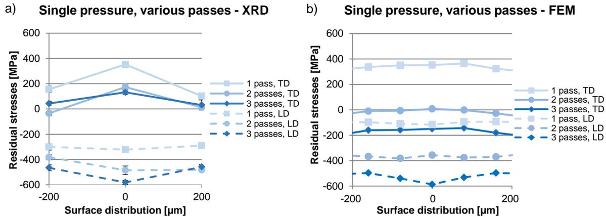
Figure 4 - Surface distribution of residual stresses transverse to the DR trace; passes variation: a) XRD measurements and b) FEM calculations
