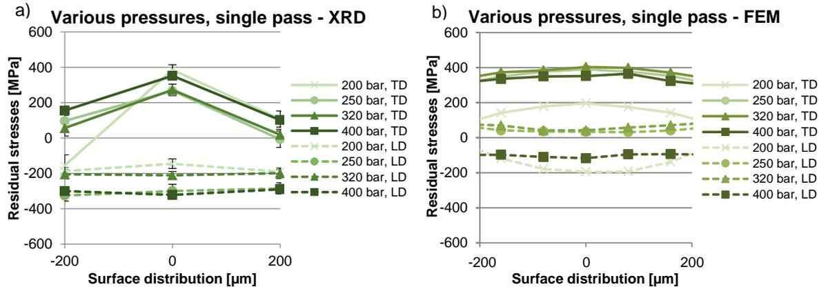
Figure 2 – Residual stresses in the center section of the DR trace for various pressures and single pass: a) XRD measurements and b) FEM calculations
