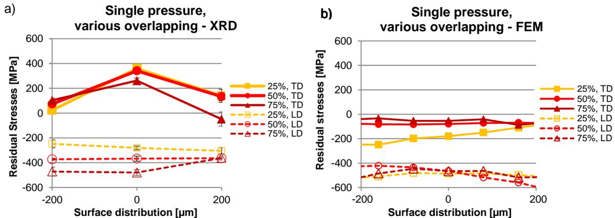
Figure 5 - Surface distribution of residual stresses transverse to the DR trace; overlapping variation: a) XRD measurements and b) FEM calculation
