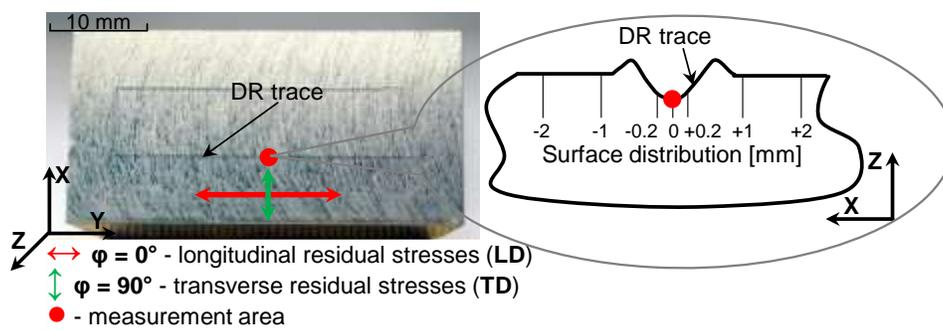
Figure 1 – geometry of the specimens and measurement area
