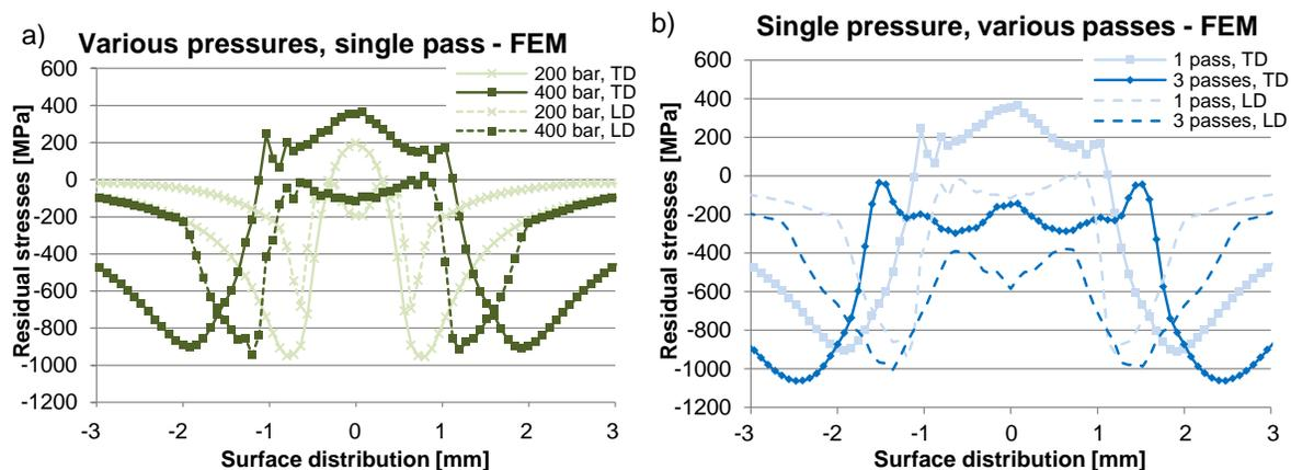
Figure 3 – Surface distribution of residual stresses transverse to the DR trace; pressure variation: a) various pressures and b) various passes
