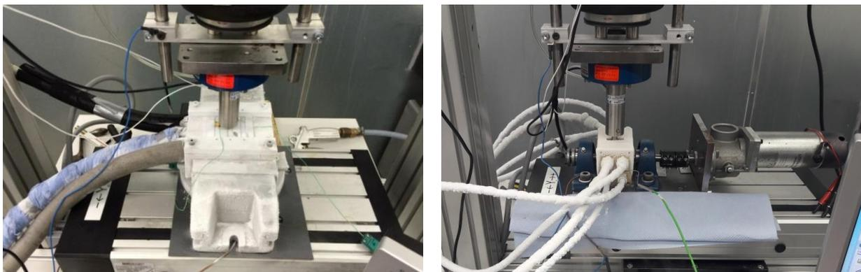
Fig. 2: Cryo PP devices for flat specimens (left) and cylindrical specimens (right)
