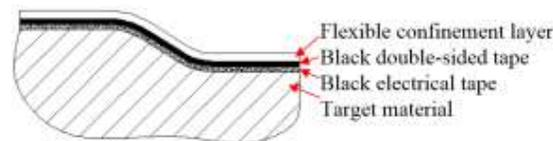
**Fig.2** Diagram of structure of the proposed flexible coating material
