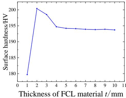
Fig.7 Strengthening effect under different thickness of FCL material
