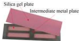
**Fig.3** Mold used for manufacturing the FCL material
