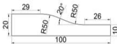
Fig.6 Curved specimen used for the continuous-impact laser shock peening
