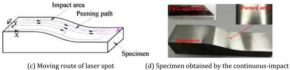
**Fig.8** Diagram of the continuous-impact laser shock peening
