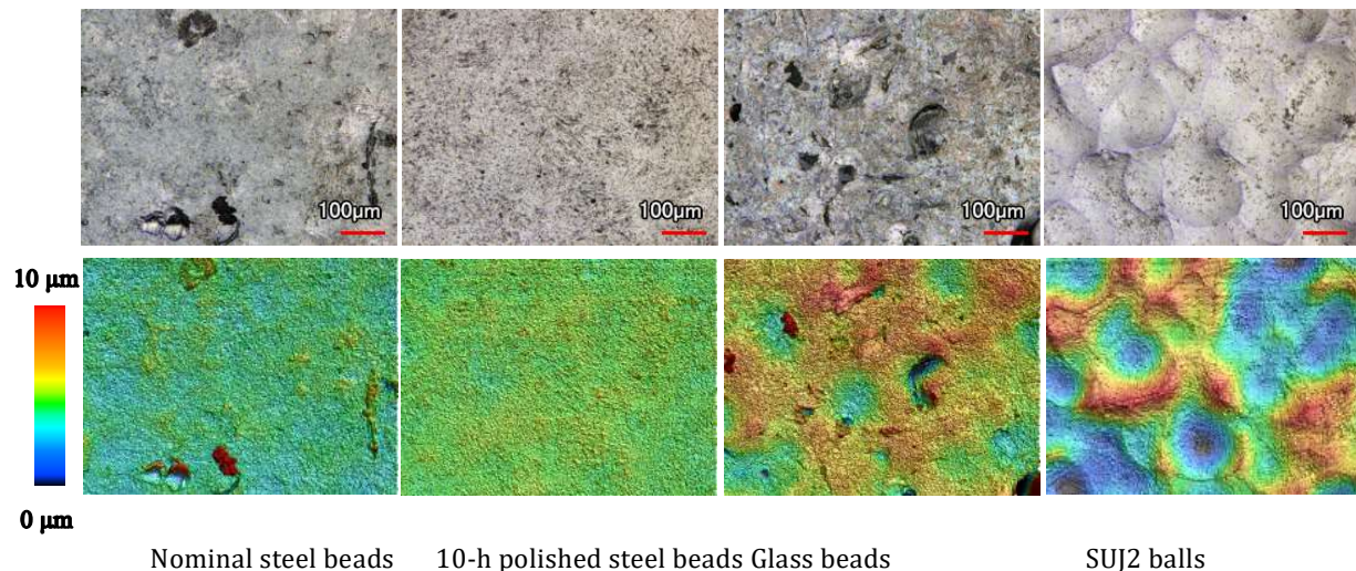
Fig. 4 Optical microscope images (upper) and surface profiles (lower) of peened surfaces
