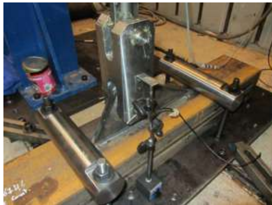
Figure 10 : Welded component tested after hammer peening repairing
