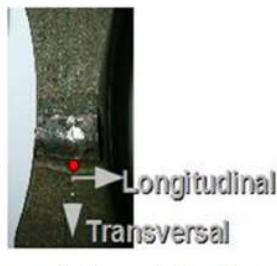
Figure 3 : Position of residual stress analyses on fatigue specimen
