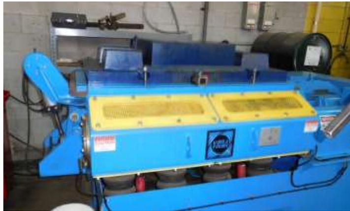
Figure 1 Vibratory peening machine at VibraFinish.
