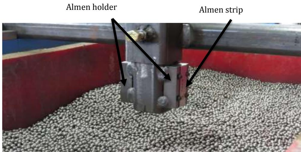
Figure 2 Vibratory peening on Almen strips for saturation test.
