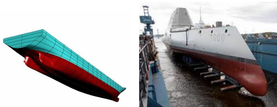
Figure 2. Open source drawing of a dual skeg ship design and photo of a ship with bulbous bow. Both structures designed to aid cruising efficiency.
