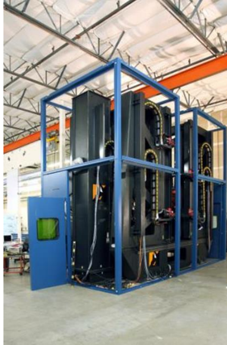
Figure 7. Prestress hardware and beam delivery system used in production laser forming since 2008.
