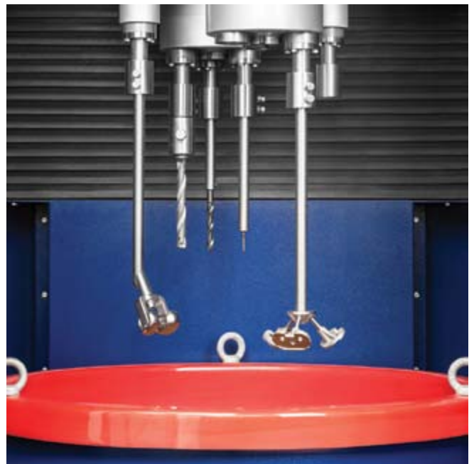
The multi-spindle heads allow up to 18 parts. Different parts were mounted onto one spindle head in this photo.
