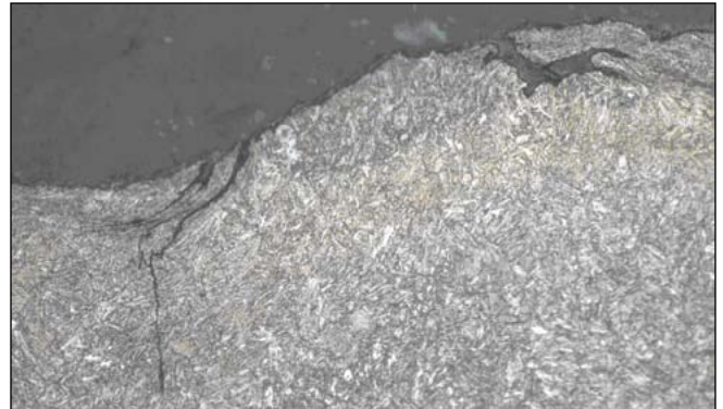
Figure 1 – Metallographically Prepared Section of Steel Leaf Spring Normal to Peened Surface after Fatigue Testing
