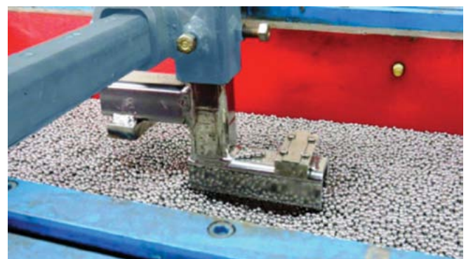
Almen strips used for process validation in a vibratory peening machine.
