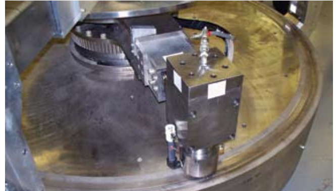
Figure 3: LPB Processing of Nuclear Waste Container Weld
