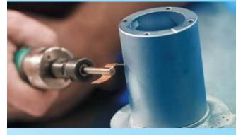
Rotary flap peening is ideal for peening small areas on new or repaired parts. The process can also be done in the field, making the time-consuming and expensive disassembly and transportation of components unnecessary.
