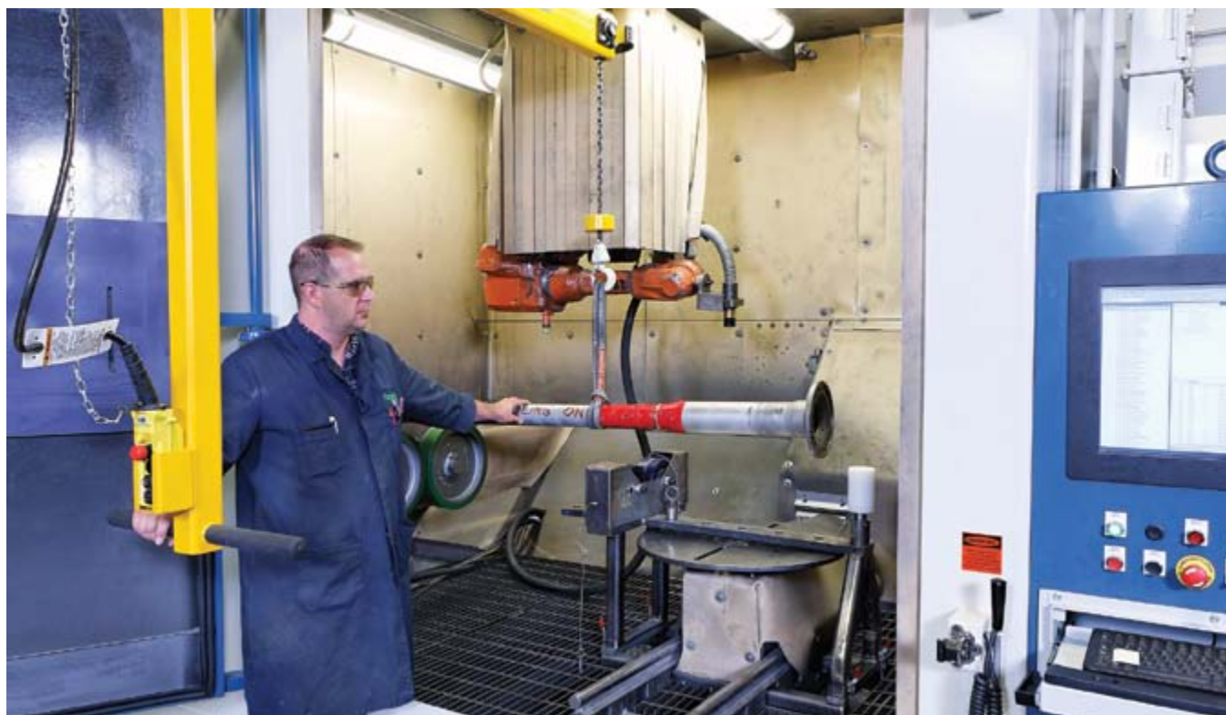
Loading a low-pressure turbine shaft for peening.
