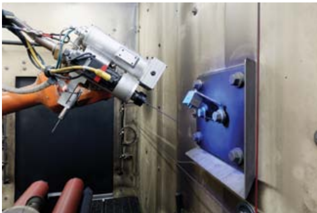
Camera locating the simulative hole in an Almen strip holder.
