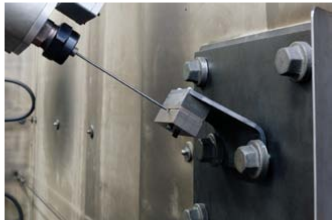
Rotary lance entering the hole of a shaded Almen strip.
