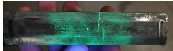
Figure 16. Corrosion-fatigue testing demonstrates the dominance of corrosion –induced cracking to lifetime. Laser peening of 23284A propulsion shaft steel sample does not fail at induced pit but eventually fails due to corrosion initiation.
