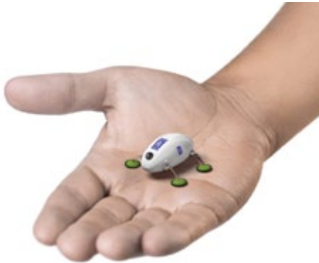
An artist's impression of the Rolls-Royce SWARM robot. The robot will crawl through engines, photographing hard-to-reach areas.
