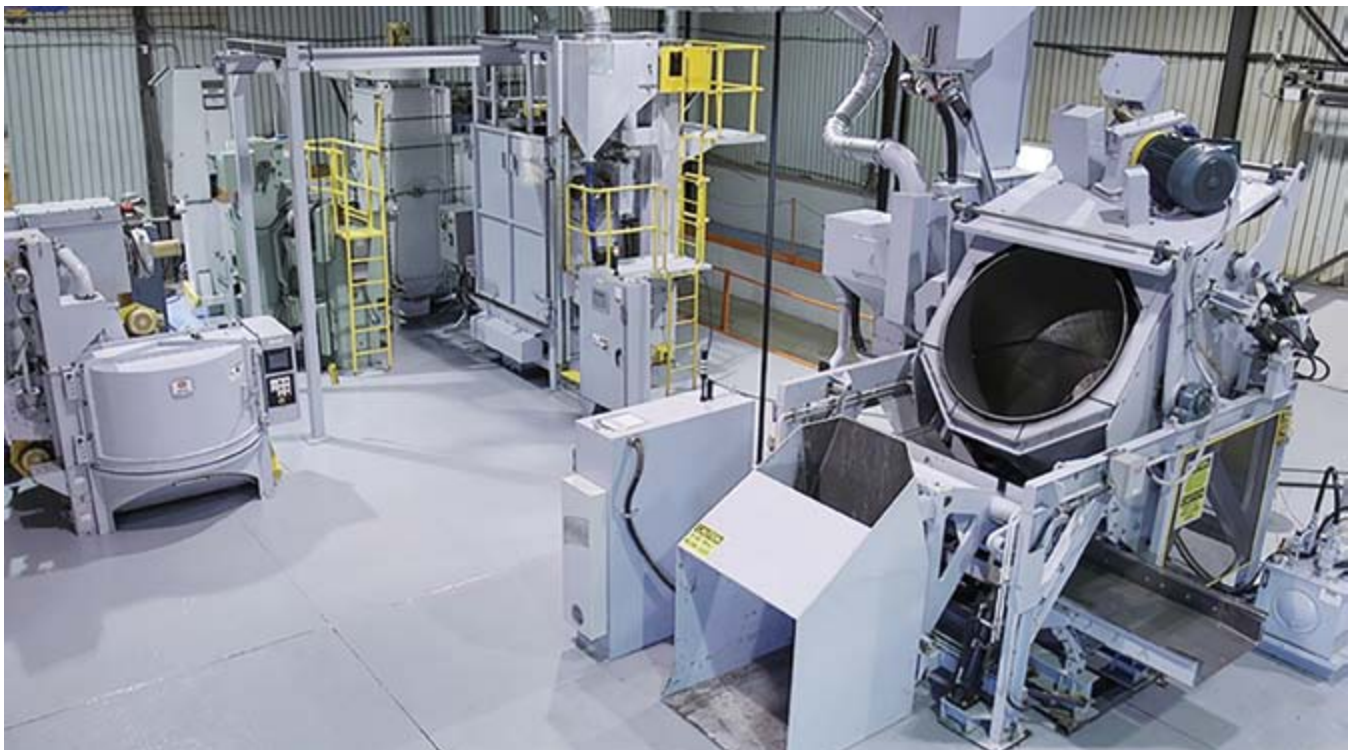
Drum shot blasting machines at Sinto America's test center in Grand Ledge, Michigan.
