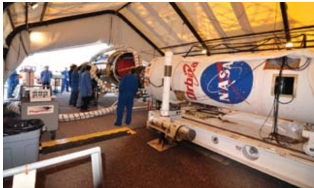
Technicians are joining NASA's Glory spacecraft with the Taurus XL rocket's third stage. The launch failed due to faulty materials from Sapa Profiles, Inc. Photo: NASA
