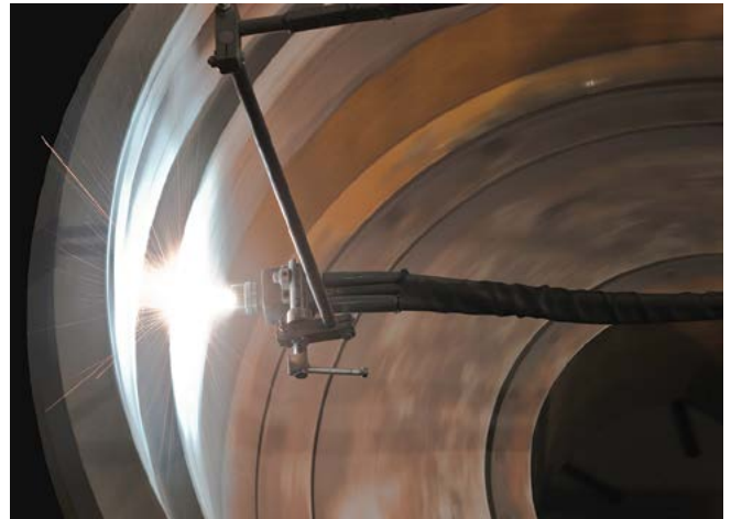
Arc Spraying on ID of Large Housing
