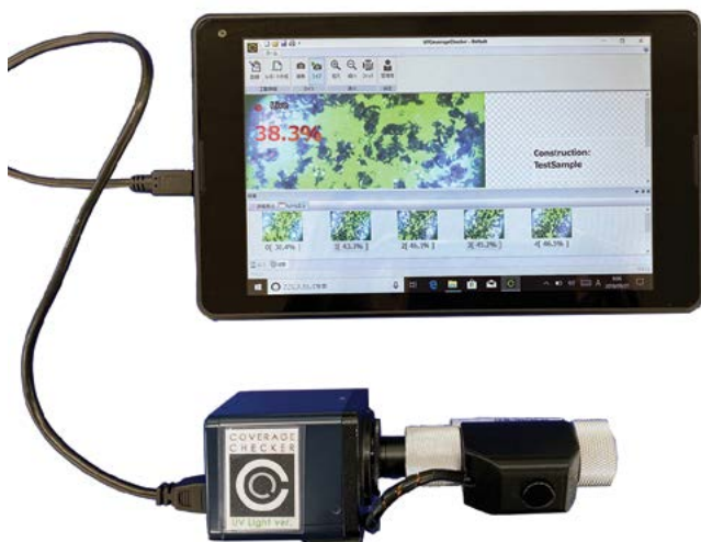
Fig. 1 Image of Coverage Checker UV light version.
