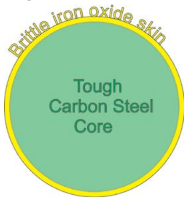
Fig.6. Iron oxide skin on carbon steel core.
